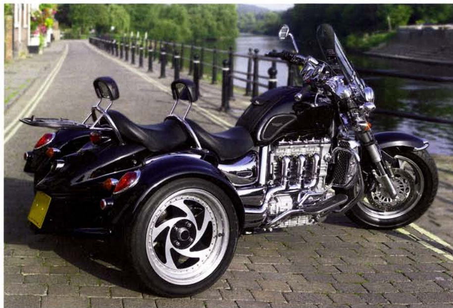
Above: the Grinnall R3T trike, £25,000, has a 150hp, 2.3 litre Triumph Rocket Three engine.
